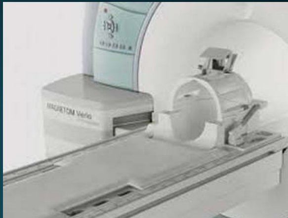
12-channel head coil with mirror for video/visual stimuli
