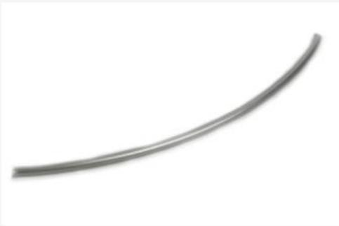
No marks on material means too low feeder tension ✗
