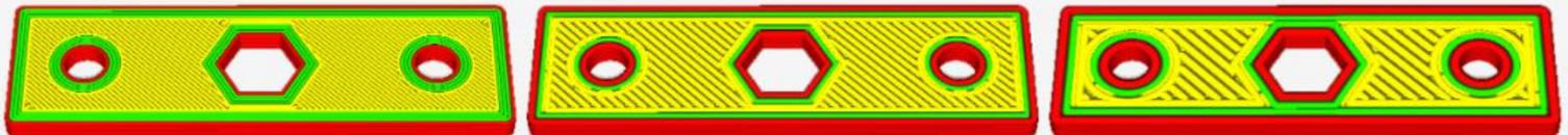
The exact same model with line widths of 0.25, 0.4 and 0.8 nozzles.
