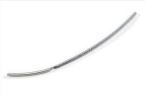
Grinding of the material means too high feeder tension ✗
